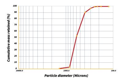
The cumulative weight percentage is illustrated in a semi-logarithmic graph where the abscissa corresponds to grain size values in logarithmic scale and full scale with the ordered values accumulated weight percentage of sand sample.
